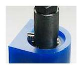
\* It is recommended that you measure the inside diameter of the hole after the first few turns to ensure that the size is accurate. Then, make any necessary adjustments to the depth of the boring bit.
