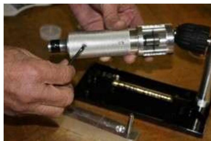
10) Snap the No. 30 HP with the holding collar on to the flex shaft. Make certain that the rotation of the blade is CCW, spinning from right to left.
