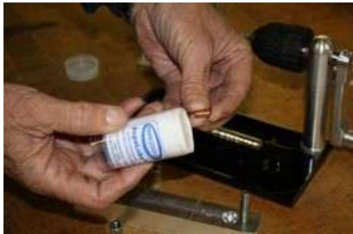
6) Place the coiled wire into the coil holding devise making certain that the lubricated side of the coil is up and the coil butts up against the stopping bracket.
