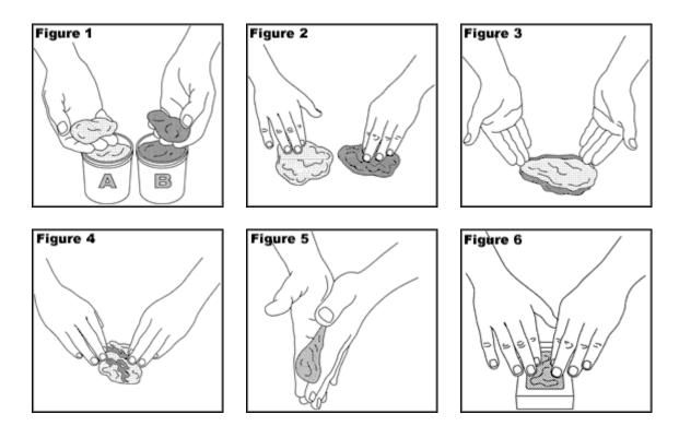
Press the mixed rubber compound into a mold frame, push the model into the rubber and then cover the model with more rubber compound. (Figure 6) A mold press, vise, clamp or heavy weight is essential to ensure that air bubbles will be driven out of the mold and one uniform piece of rubber is created.
